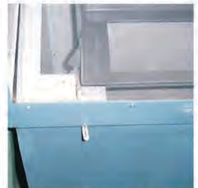
Crucible mixer with carriage lock in place. Door cannot fully close and cannot engage the door interlock.
